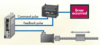
Simplified Synchronization: It is also possible to input encoder output signals directly into the servo drive.
