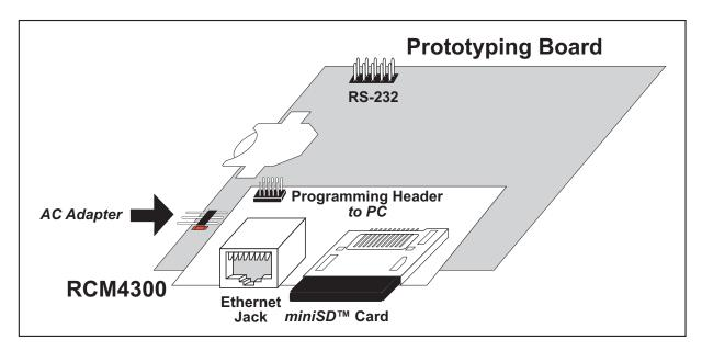
Figure 1. Application Kit Setup
