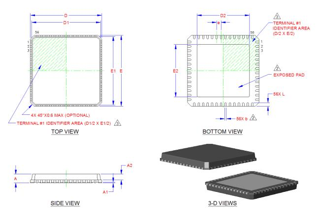
Figure 2 56-QFN Package Definition
