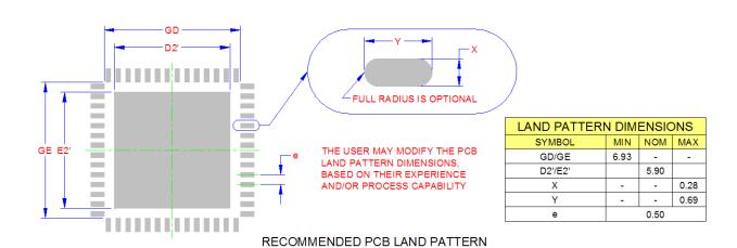
Figure 3 56-QFN Recommended PCB Land Pattern
