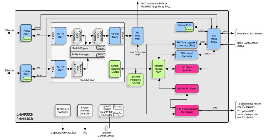
Figure 1 Internal Block Diagram
