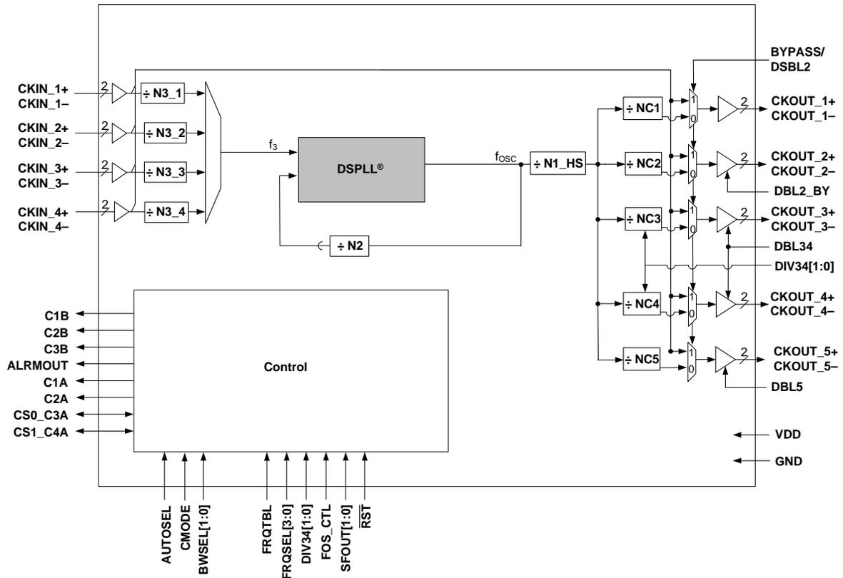
**Figure 9. Si5365 Low Jitter Clock Multiplier Block Diagram**
