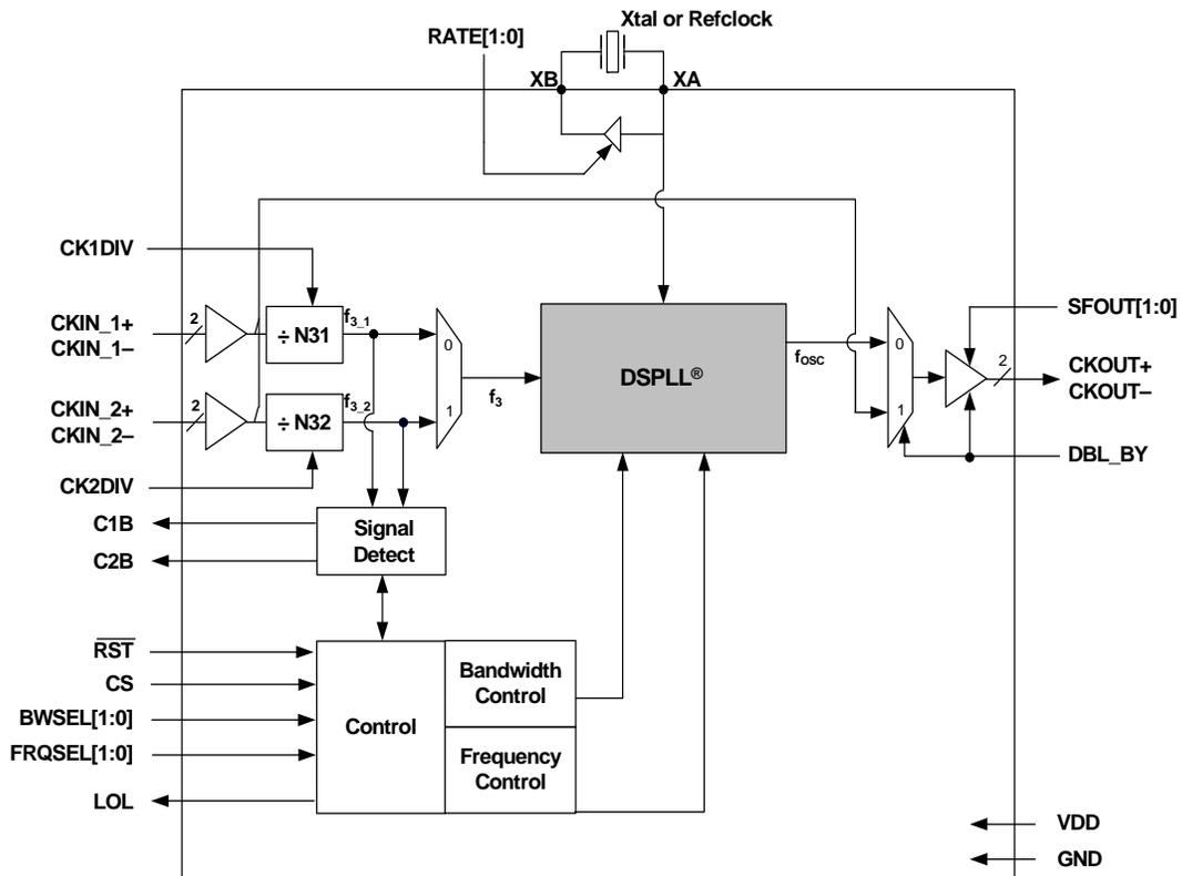
Figure 1. Si5316 Any-Frequency Jitter Attenuator Block Diagram
