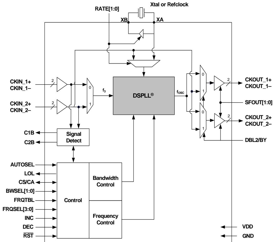
Figure 4. Si5323 Jitter Attenuating Clock Multiplier Block Diagram
