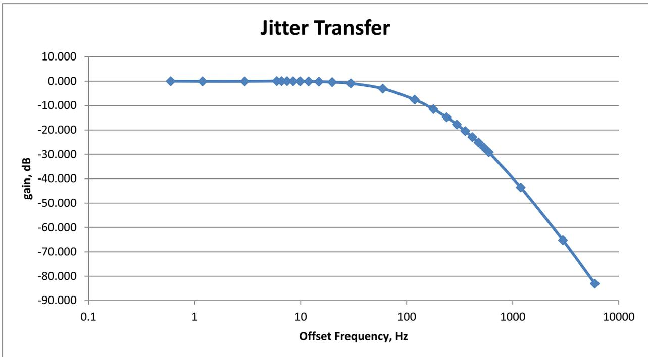
Figure 106. Wide View of Jitter Transfer
