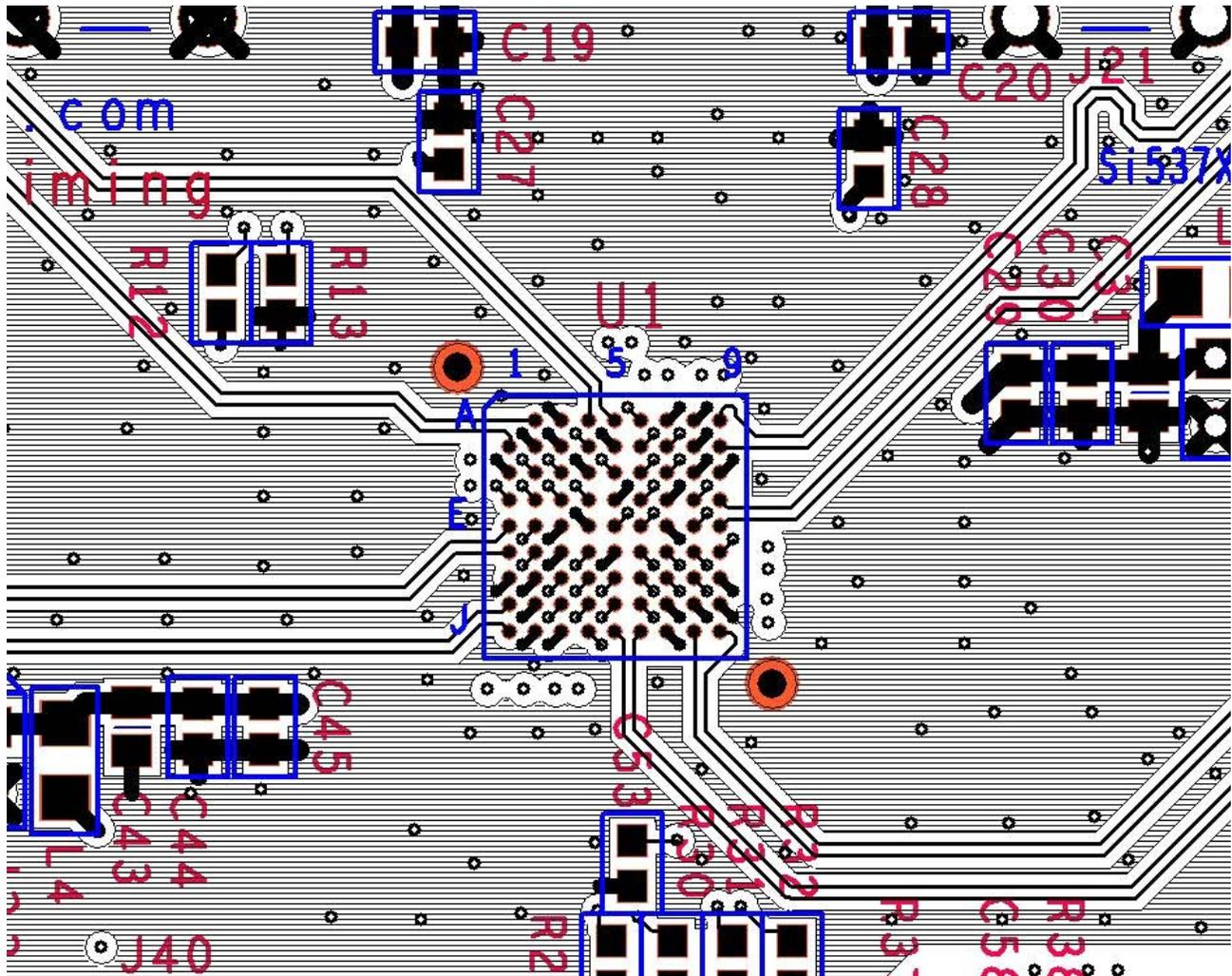
**As much as is possible, do not route clock input and output signals underneath the BGA package. The clock output signals should go directly outwards from the BGA footprint.**
