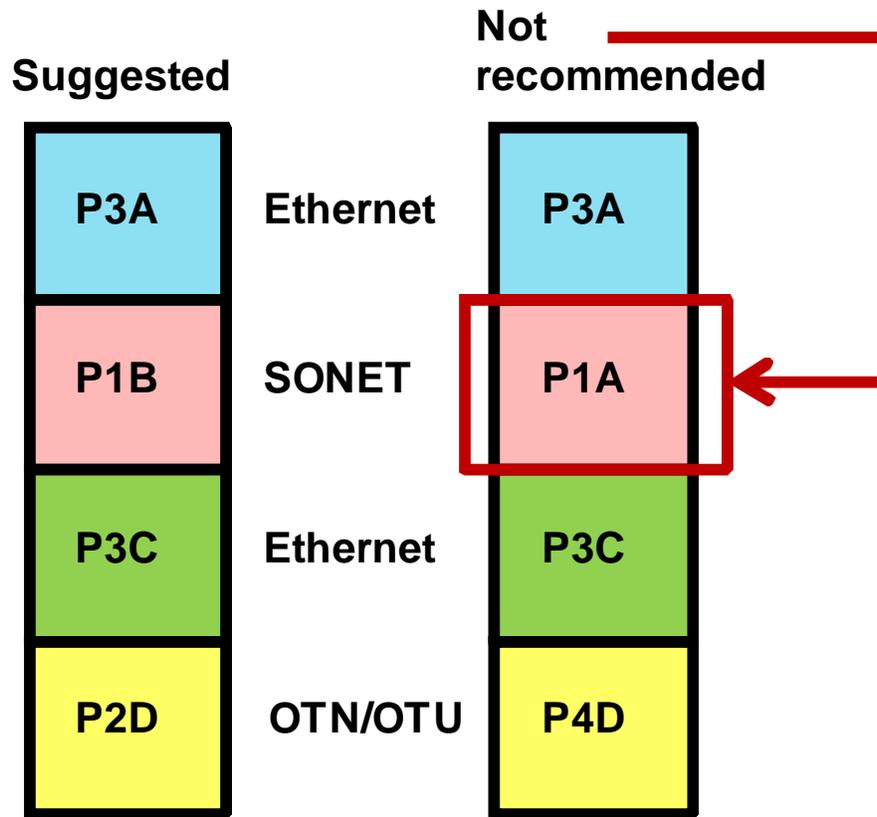
Figure 105. Run Time Frequency Plan Examples
