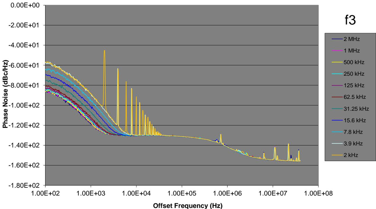
Figure 58. Phase Noise vs. f3
