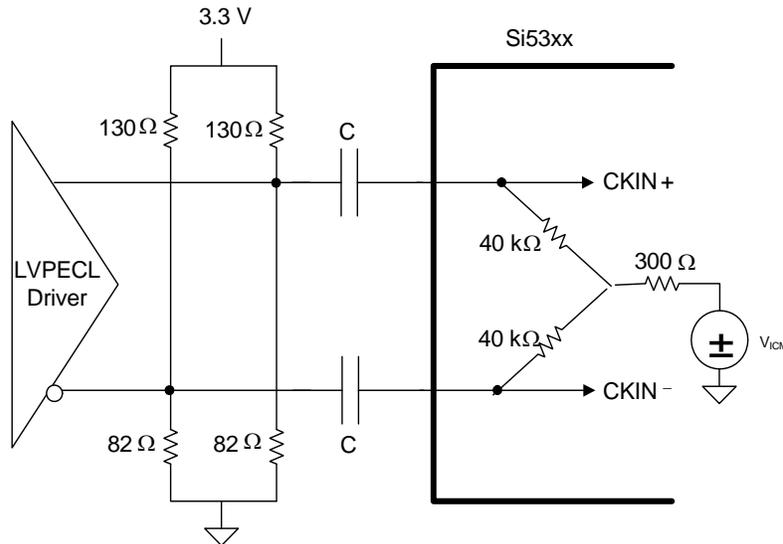
**Figure 36. Differential LVPECL Termination**
