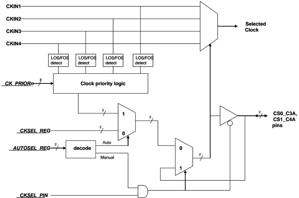
**Figure 25. Si5367, Si5368, and Si5369 Input Clock Selection**
