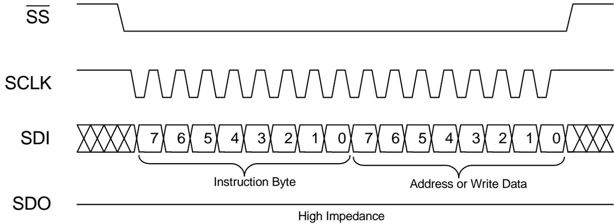
**Figure 33. SPI Write/Set Address Command**
