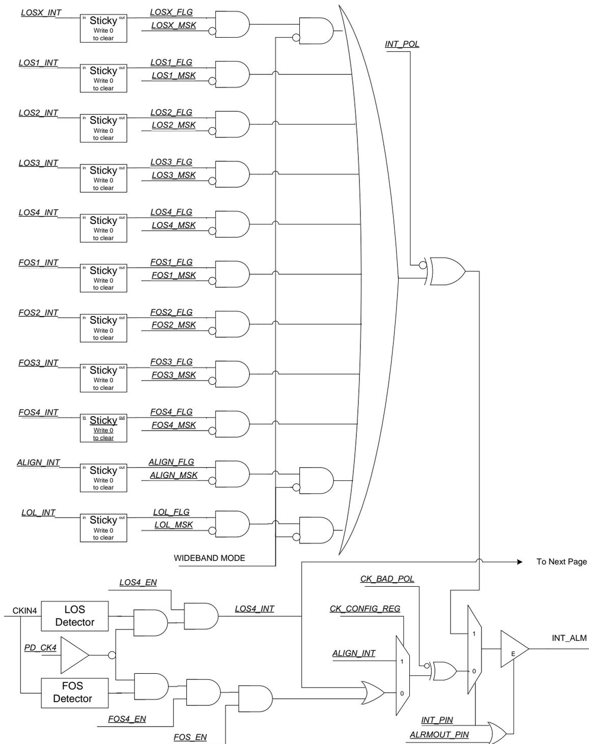
Figure 83. Si5368 and Si5369 Alarm Diagram (1 of 2)
