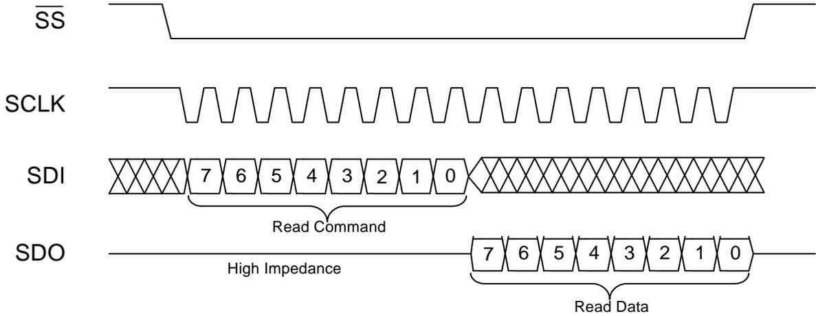
**Figure 34. SPI Read Command**
