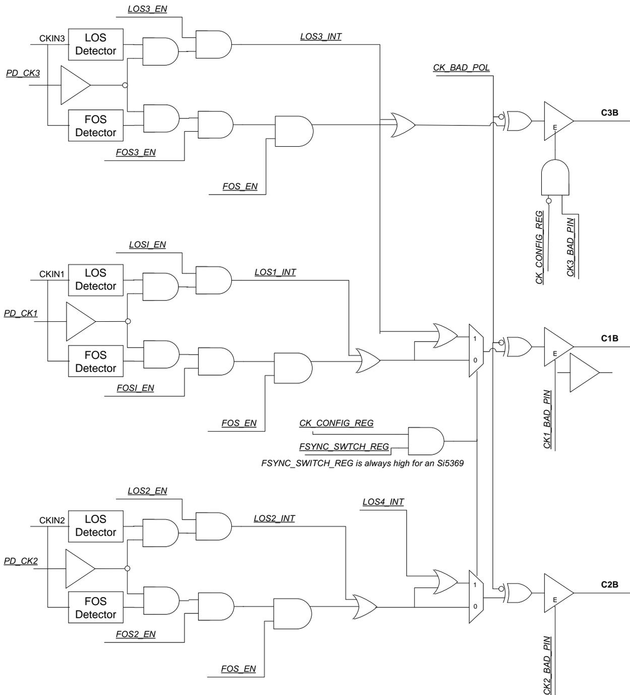
Figure 84. Si5368 and Si5369 Alarm Diagram (2 of 2)
