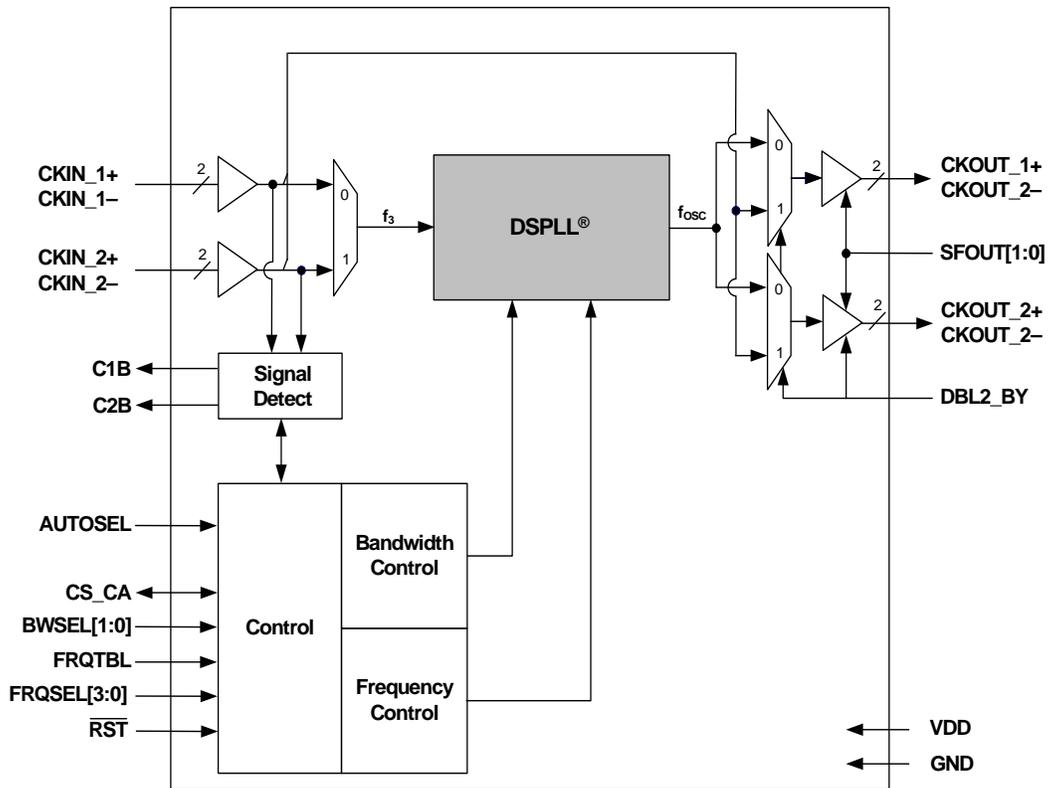
Figure 3. Si5322 Low Jitter Clock Multiplier Block Diagram
