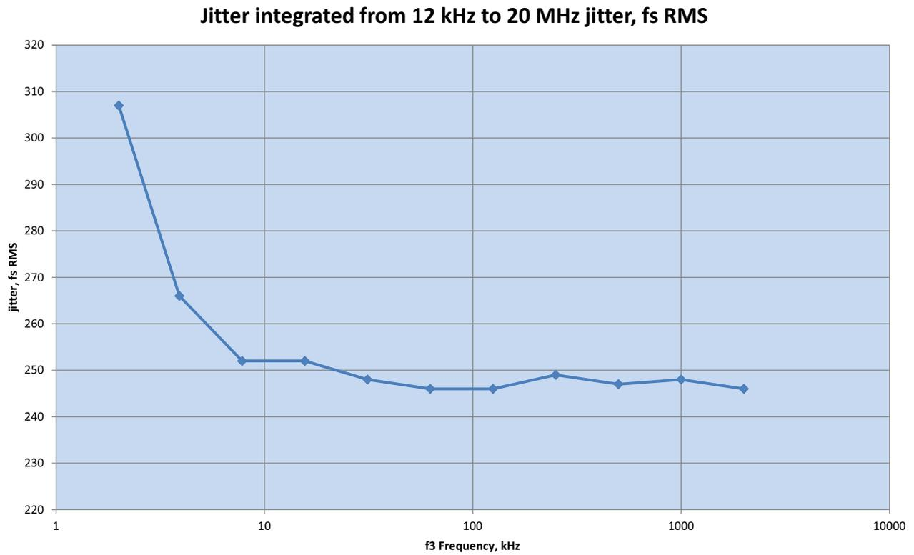
Si5326, LVPECL,  $V_{dd}=3.3V$ ; brick wall integration
