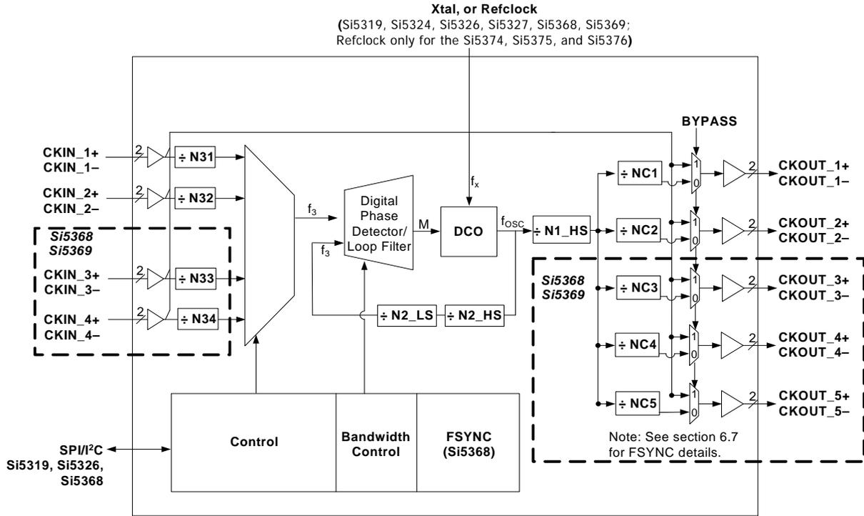
Note: There are multiple outputs at different frequencies because of limitations caused by the DCO and N1\_HS.
