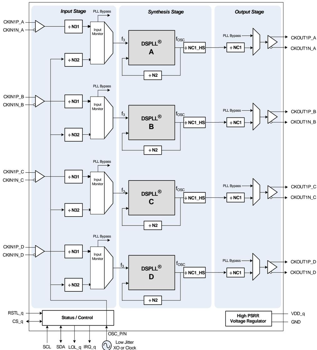
Figure 15. Si5375 Functional Block Diagram
