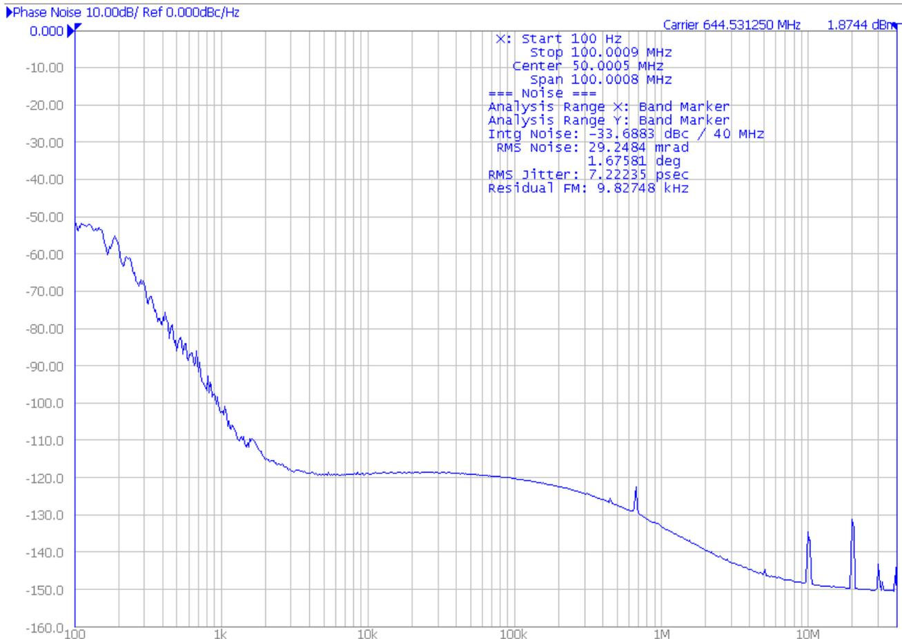
**Figure 74. 78.125 MHz In; 644.531 MHz Out**
