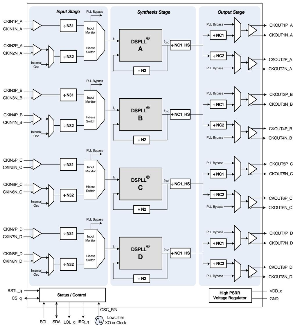
Figure 16. Si5376 Functional Block Diagram
