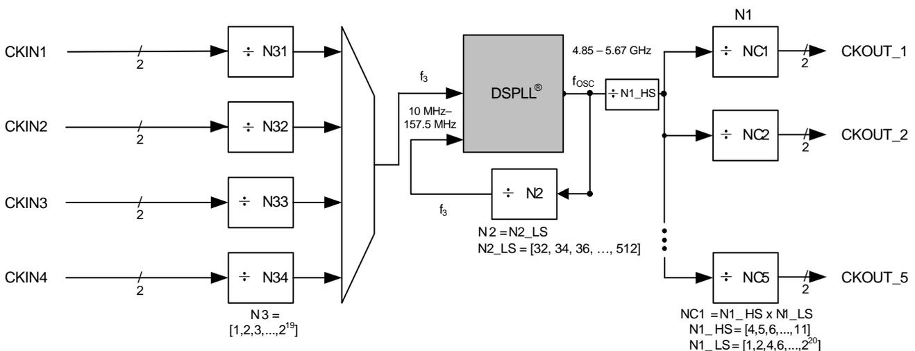
Figure 22. Wideband PLL Divider Settings (Si5325, Si5367)
