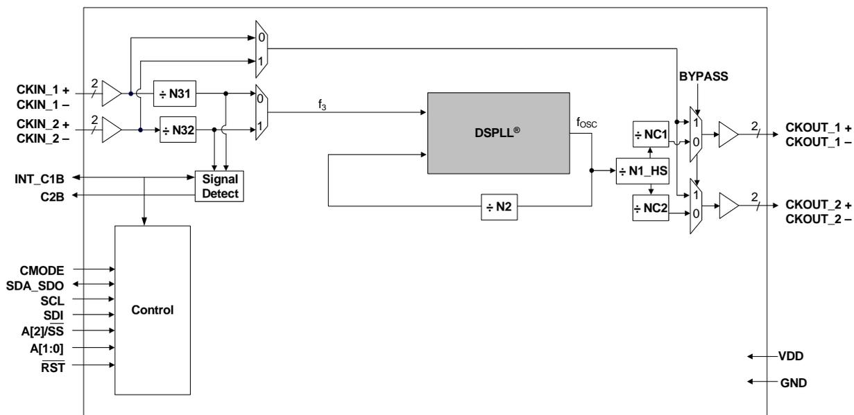
**Figure 6. Si5325 Low Jitter Clock Multiplier Block Diagram**
