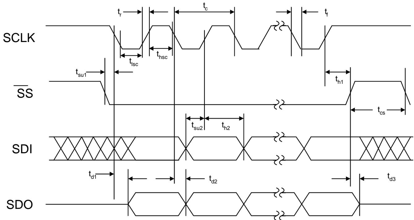
Figure 35. SPI Timing Diagram
