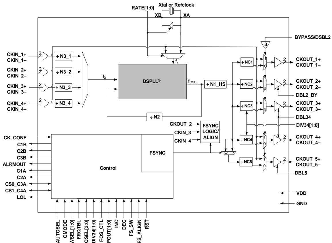
Figure 10. Si5366 Jitter Attenuating Clock Multiplier Block Diagram
