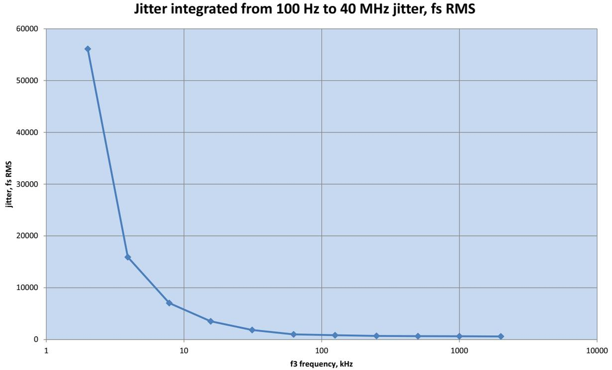
Si5326, LVPECL,  $V_{dd}=3.3V$ ; brick wall integration
