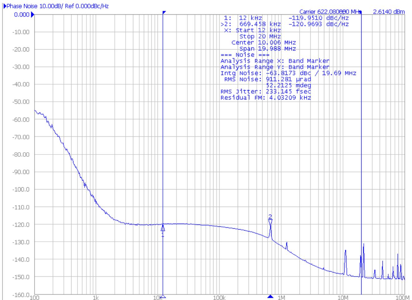
Figure 65. 155.52 MHz In; 622.08 MHz Out
