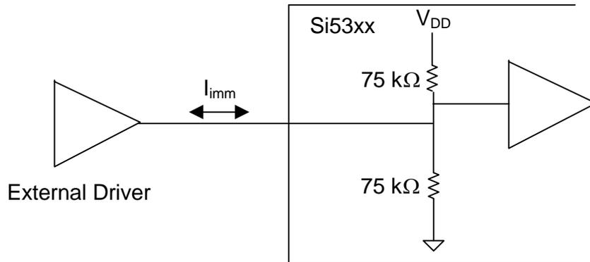
Figure 53. Three Level Input Pins
