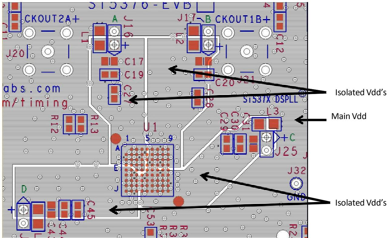
The four Vdd supplies should be isolated from one another with four ferrite beads. They should be separately bypassed with capacitors that are located very close to the Si537x device.
