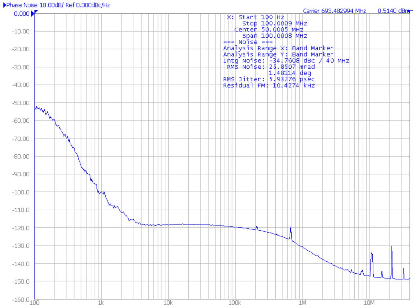
**Figure 76. 78.125 MHz In; 693.493 MHz Out**
