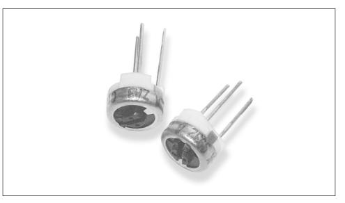
For applications that demand a durable, miniature trimming potentiometer, this military style offers quality at the right price. Cermet element technology ensures stability and performance in these 6mm diameter components. All units are fully sealed to withstand immersion in normal board washing solvents.
