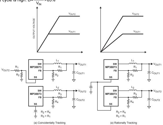
Figure 6—Output Voltage Tracking
