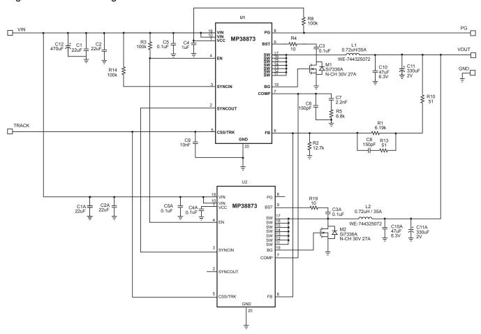
Figure 7—Two Phase Operation
