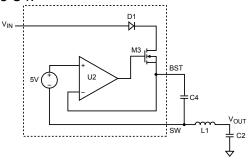
Figure 3—Internal Bootstrap Charging Circuit Startup and Shutdown
