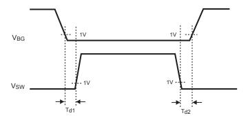
Figure 1—Gate Drive Non-Overlap Time Diagram
