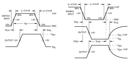
FIGURE 2. AC Waveforms
