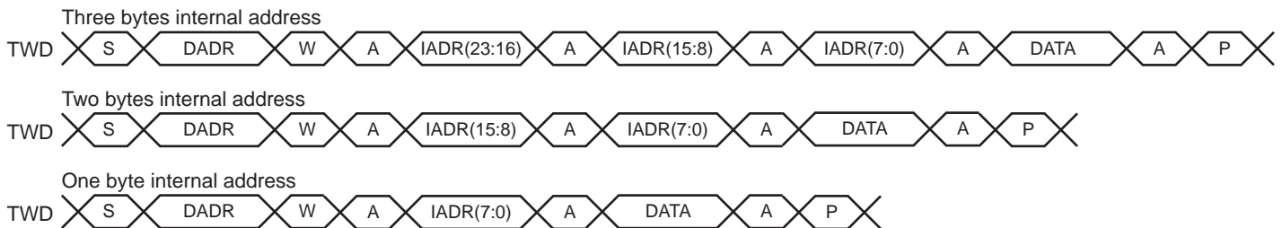
Figure 32-10. Master Write with One, Two or Three Bytes Internal Address and One Data Byte
